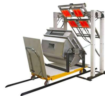
Roofing Test with Two Stages incorporating Burning Brands, Wind and Supplementary Radiant Heat – EN 1187 Test 4
