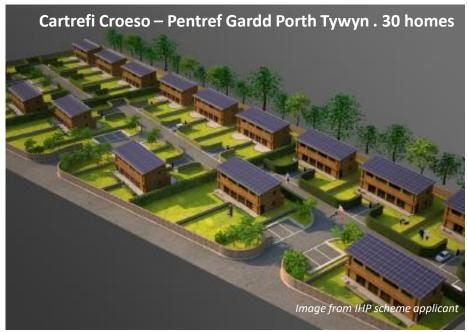
Innovation: Panalised, using Ty Solar system, external larch clad, spruce framing. Local factory potential to supply 100 homes per annum, local labour
